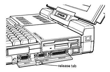
4. One end of the printer cable has a 25-pin, D-shaped male connector. (See your printer manual if you cannot identify this connector.) Connect this end to the parallel connector labeled PRINTER on the right side of the computer, as shown below. If the plug has retaining screws, tighten them by hand or with a screwdriver.
